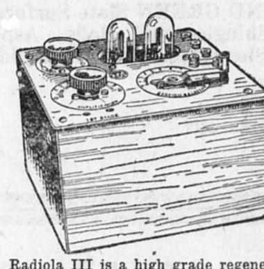
Radiola III is a high grade regenerative broadcast receiver employing two Radiotrons WD-11. One stage of audio frequency amplification is provided, utilising improved transformers for purer amplification.
