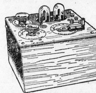
Radiola III is a high grade regenerative broadcast receiver employing two Radiotrons WD-11. One stage of audio frequency amplification is provided, utilising improved transformers
