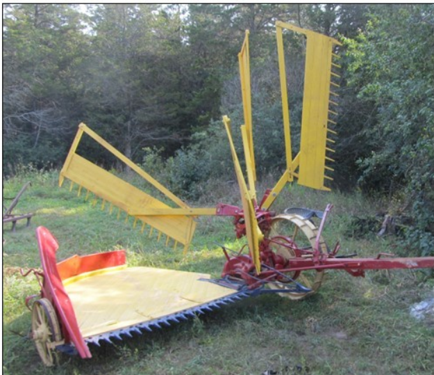
McCormick Reaper, circa 1850-1875 Cuts grain and leaves in bundles
