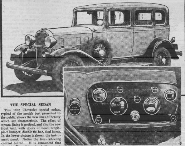
the 1932 Chevrolet engine is 20 per cent. greater in power and there are many of which is the combination of syncro- wheeling for the first time in any car as other mechanical improvements, the chief mesh transmission with simplified free- standard equipment.
