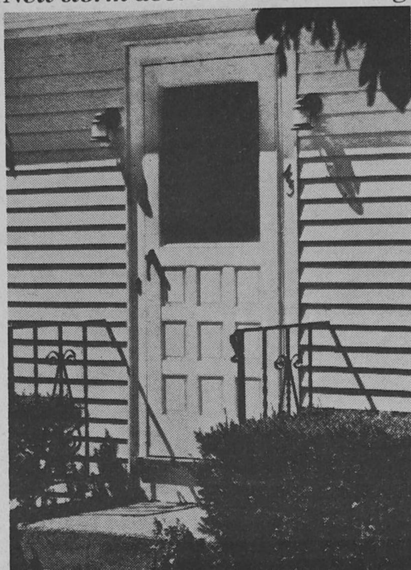
CONSTRUCTED OF structural foam polystyrene with inner metal reinforcements, the new Woodstead™ summer/winter storm door resists constant wear and tear in all types of weather. Weighing only 38 lbs., the door by building materials manufacturer, Bird & Son, inc., East Walpole, Mass., can be easily installed by one person. An attractive wood grain texture and raised panels make the Woodstead™ storm door a distinctive addition to any home.
