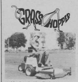
Hydrostatic Drive · Zero Turning Radius for Unlimited Maneuver · Complete Speed and
