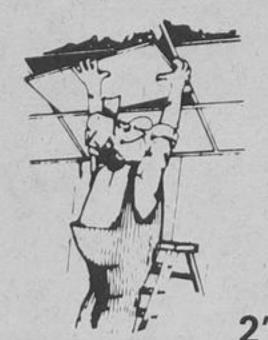
This system for ceilings is ideal for lowering high ceilings, hiding water and heating pipes, ductwork, etc. The steel grid system is easy to install, and has a baked white enamel finish.
