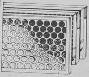
A dirt clogged furnace filter makes it hard for your furnace to heat your home. Change it now before the cold weather sets in and save fuel by replacing it often.
