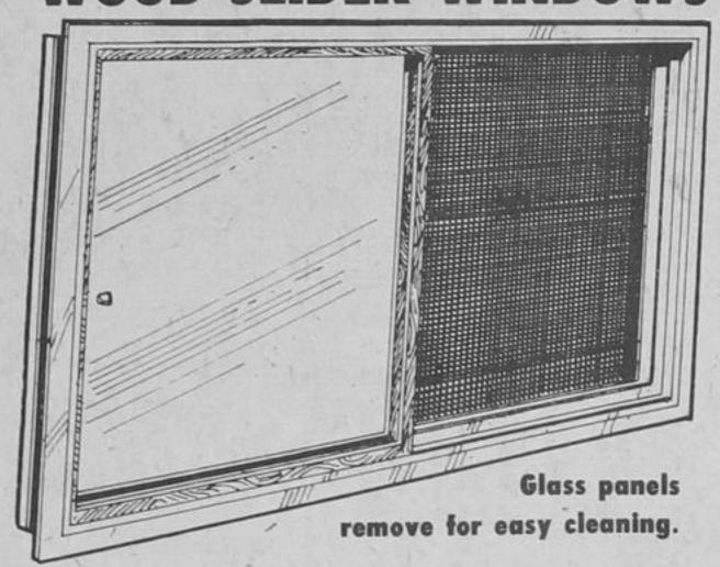
Two wood frames hold the glass panels which bypass smoothly in a white vinyl sill and pressurized top header. Rigid and soft vinyl-weatherstripping at the side jambs and meeting rail provides the ultimate in weather tightness.
