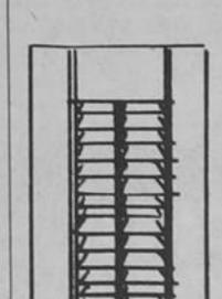
STILES: 13/16" Thick x 1-9/16" TOP RAILS: 5/8" thick x 3" BOTTOM RAILS: 5/8" thick x 2-7/8". All panels can be trimmed as much as 1" in width and 4" in height
