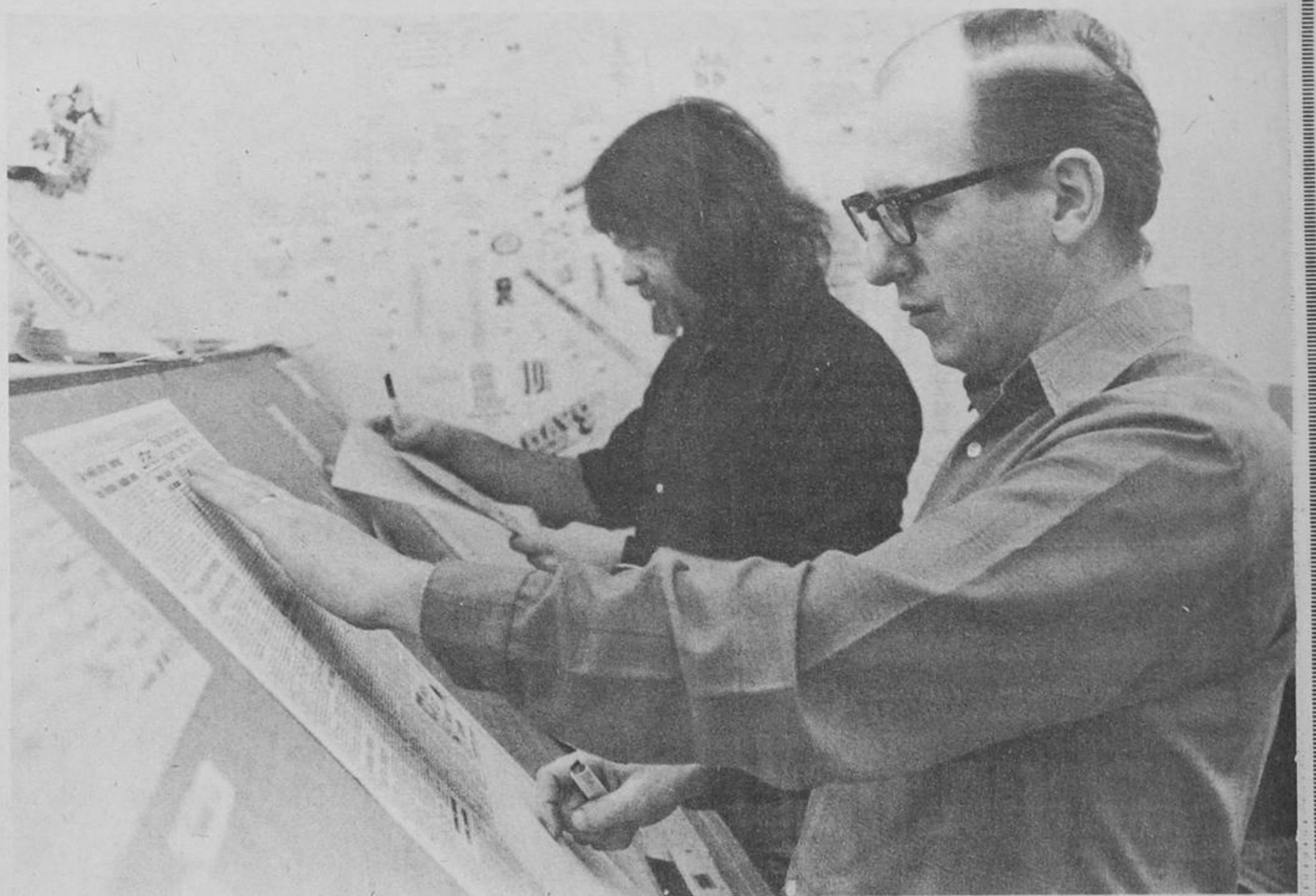
Veteran linotype operator, Ed Lloyd, (foreground), and Dave Belanger paste waxed copy on layout sheets. The layout sheets, or page flats, go to Newsweb Enterprise Limited in Willowdale, where they are photographed. From the negative, a plate is made to go directly onto the press.
