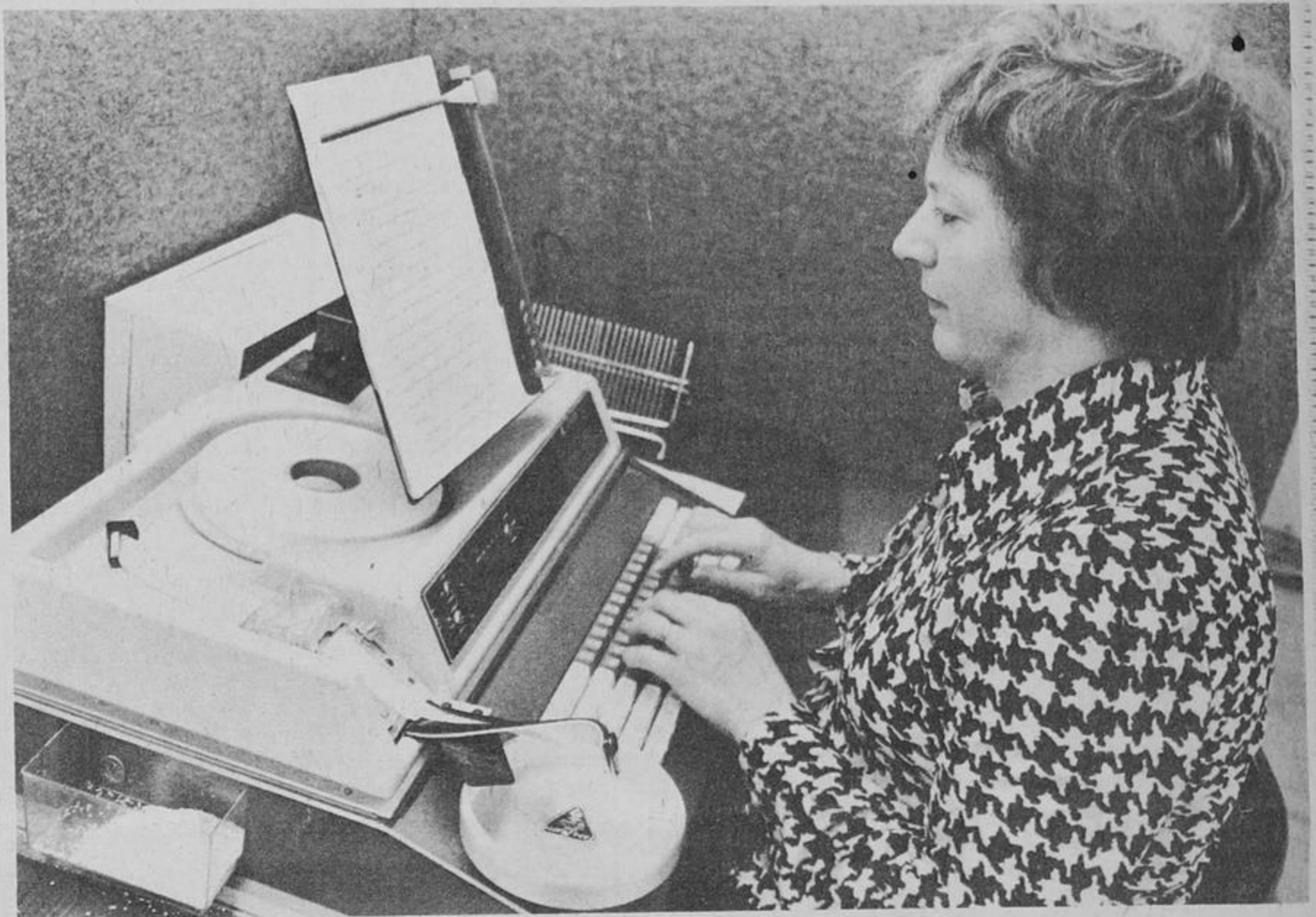
Eileen Mitchell, one of the composing room typesetters, follows copy from The Liberal editorial office and types it on her keyboard. The result — a punched tape — can be seen flowing into the circular dish on the left. A little plastic box on the side of the machine catches the perforated pieces from the tape.
