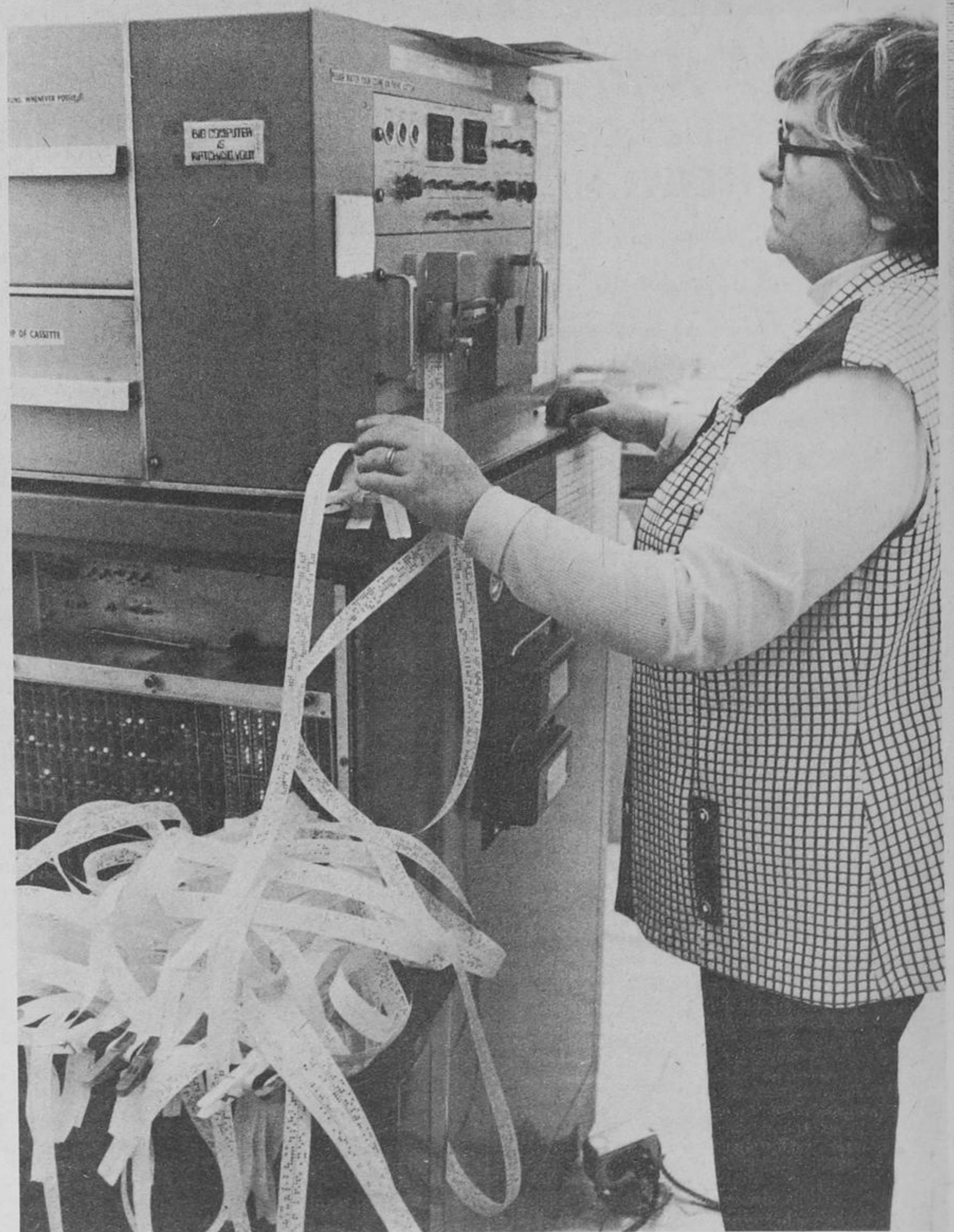
Typesetter Jean St. John watches a tape roll off the Compugraphic 4961 in Aurora. The computer reads the tape and a light flashing through a spinning cellulose "font" prints the letters on photographic
