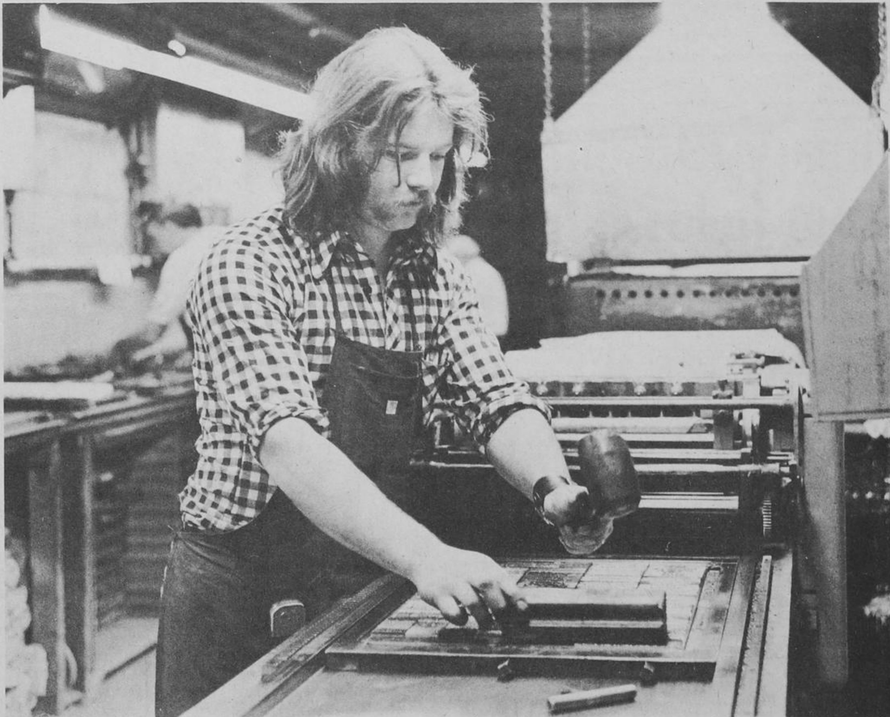
David Belanger, employed at The Liberal for two years, uses a wooden block and rubber mallet to level the type on the proof press. A paper mache impression of the surface was made under a
