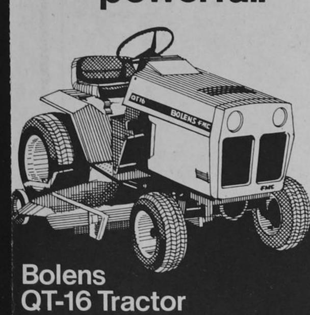
The irritating noise and vibration are gone. The rugged workpower remains. Powerful 16 horse, twin cylinder engine. Precise, uncomplicated controls. A power-locking collar clicks attachments in line with just fingertip pressure. One treadle-pedal controls speed and direction. Attachment clutch and hydraulic lift are flip switches, not arm-wrenching levers. Someday, all tractors will be this sophisti-
