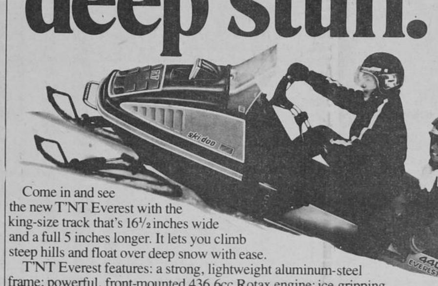
frame; powerful, front-mounted 436.6cc Rotax engine; ice-gripping carbide ski runners; and speedometer, tach, tripometer and shock absorbers. as standard equipment. And, of course, a full one year warranty.
