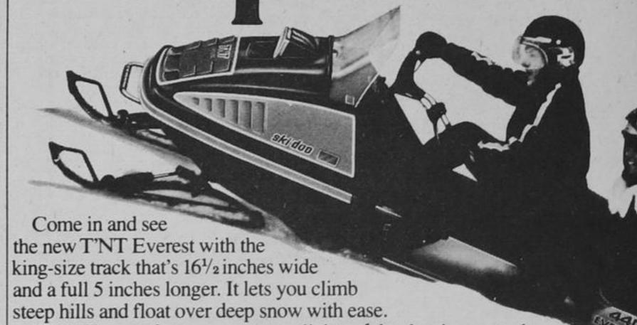
T'NT Everest features: a strong, lightweight aluminum-steel frame; powerful, front-mounted 436.6cc Rotax engine; ice-gripping carbide ski runners; and speedometer, tach, tripometer and shock absorbers.
