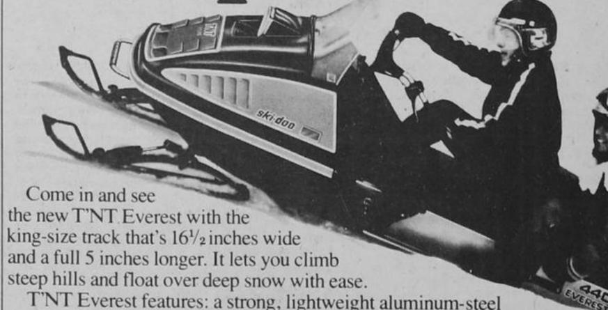
T'NT Everest features: a strong, lightweight aluminum-steel frame; powerful, front-mounted 436.6cc Rotax engine; ice-gripping carbide ski runners; and speedometer, tach, tripometer and shock absorbers. as standard equipment. And, of course, a full one year warranty.
