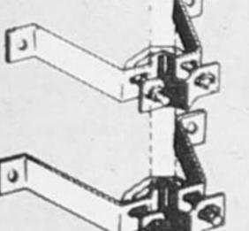
4" Wall Mounts · Holds Mast 4" From Wall
