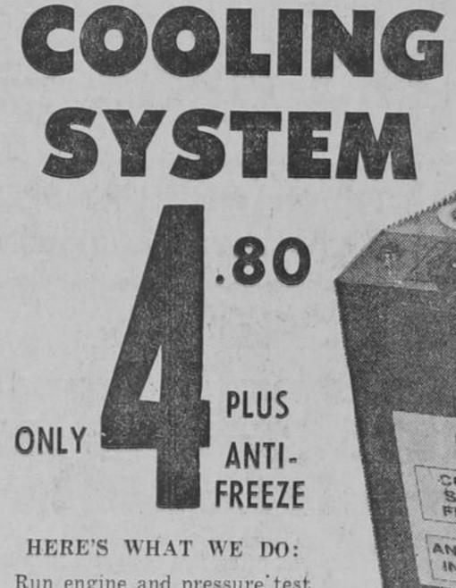
Run engine and pressure test system for leaks, test cap pressure, tighten hose connections and belt tension, drain radiator, flush complete system and fill with anti-freeze, using our modern flush and fill machine. Check dash instrumentation.
