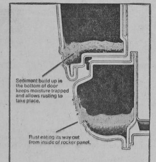
The most dangerous rust begins in the hidden boxed in areas of your car. This diagram shows cross section of a door and rocker panel being attacked by rust.
