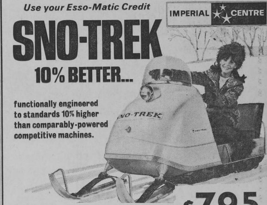
Steel reinforced endless rubber track with double centre sprocket drive-10% less power loss, less wear.
