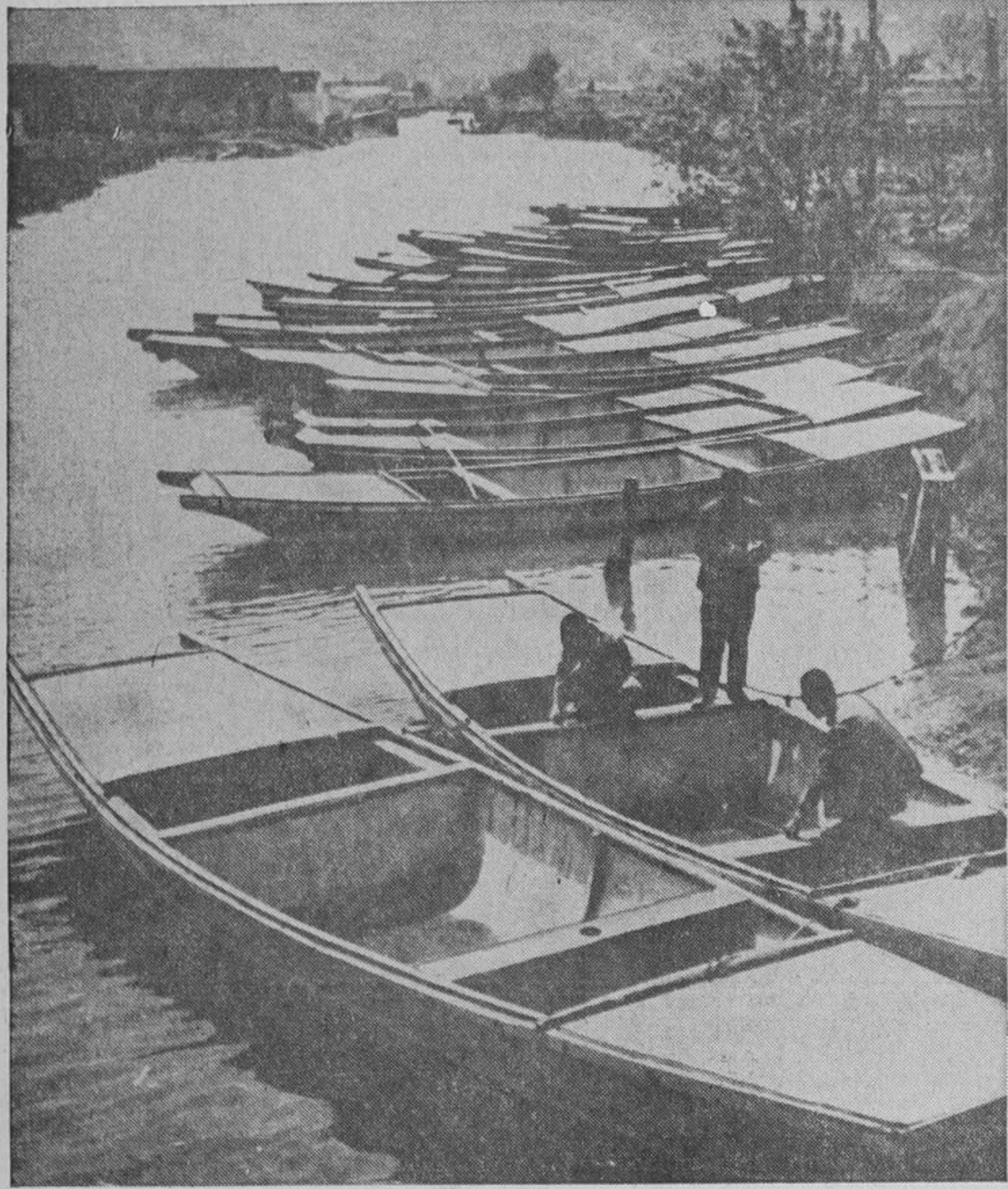
CEMENT BOATS —Cement boats with wire frames were built by the Wuhsi shipyard in Kiangsu Province, Communist China, for use in rural areas of east China.
