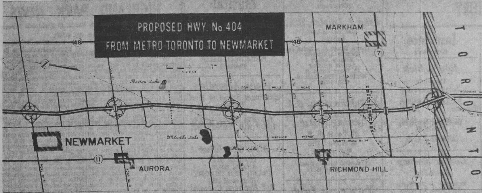
Proposed route of a new four-lane controlled-access highway to connect with the Don Valley Parkway at the northern limits of Metro and running north to the vicinity of Newmarket is shown above. This will be the first stage of the freeway which the Department of Highways proposes to build eventually to the area east of Lake Simcoe. Details of the proposed route, timing of property purchase and highway construction (still several years away) and other details
