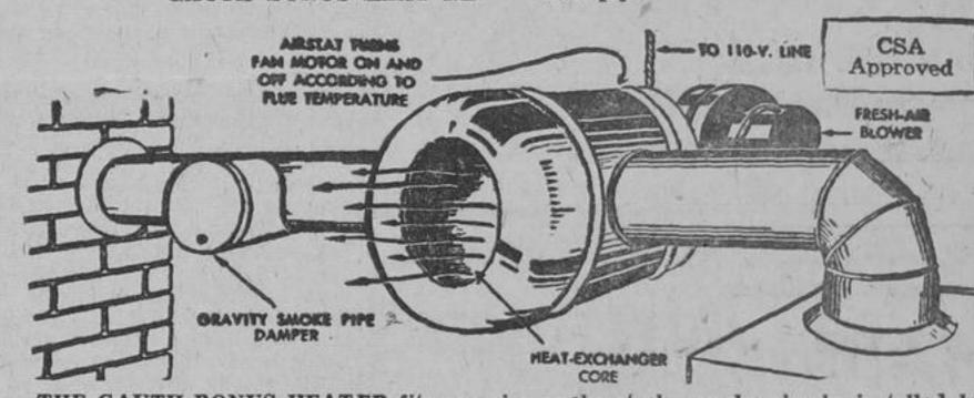
THE GAUTH BONUS HEATER fits any size smoke stack can be simply installed by most homeowners, as it will easily fit into as small as 12 inches of smoke stack, with a heat loss of as low as 450 degrees. Weight only 11 lbs. Guaranteed satisfaction or money refunded. EASY TERMS
