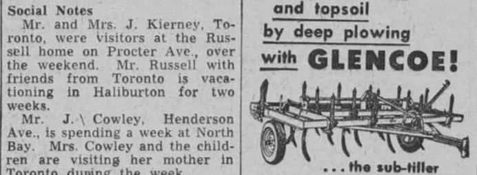
with fast power lift The rugged Glencoe sub-tiller plow breaks up the hardpan, allowing moisture to be absorbed faster and deeper. The exclusive power lift (or alternative hydraulic lift) enables the plow to be raised or lowered, instantly-from the tractor seat. Penetration may be set at any depth up to 14". Each shank has strong double springs for fast, trouble free clearance of obstacles.
