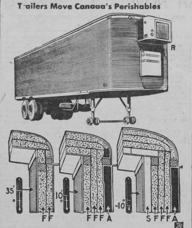
Canada's perishable food supply is moving over the highway in mechanically refrigerated stainless steel trailers. As a result farm products are reaching Canadian tables fresher and more palatable. Food products are transported at proper temperatures. Frozen foods, for example, have to be kept as low as 10 degrees below zero, say Fruehauf Trailer company engineers. Glass fiber insulation has been very helpful because it keeps the
