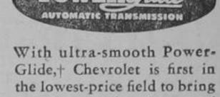
you the proudest feature of luxury cars - a fully-proved, fully-automatic transmission. There's no clutch pedal! You can drive all day without ever shifting a gear! And with all this driving ease, you get the extra-abundant power of Chevrolet's new 105 h.p. engine, exclusive to PowerGlide Chevrolets. It's so simple to drive, it's a thrill to drive!
