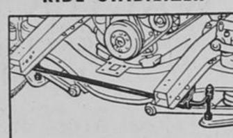
Attached to the front end of the chassis frame, and linked to the lower Knee-Action member, it imparts genuine steadiness on curves and sharp turns!
