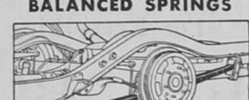
With double-acting shock absorbers, and with spring action varying automatically according to load and deflection, "balanced springing" assures uniform riding smoothness.
