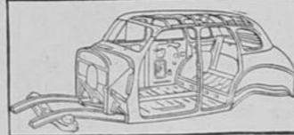
The strongest and most rigid body and frame construction known to modern automotive engineeringmakes for solid, long-lasting comfort and safety.
