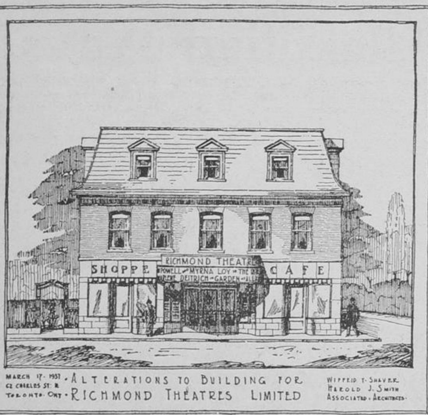
The above shows architects' drawing of the proposed new Richmond Theatre, Richmond Hill. It is proposed to remodel the present hotel building at Yonge and Arnold Streets into two modern stores with four living apartments on the upper floors. The entrance to the theatre which will be constructed at the rear will be on Yonge Street between the stores as shown in drawing. The project is sponsored by a local company, Richmond Theatres Limited, and stock in company is now being offered to the public.
