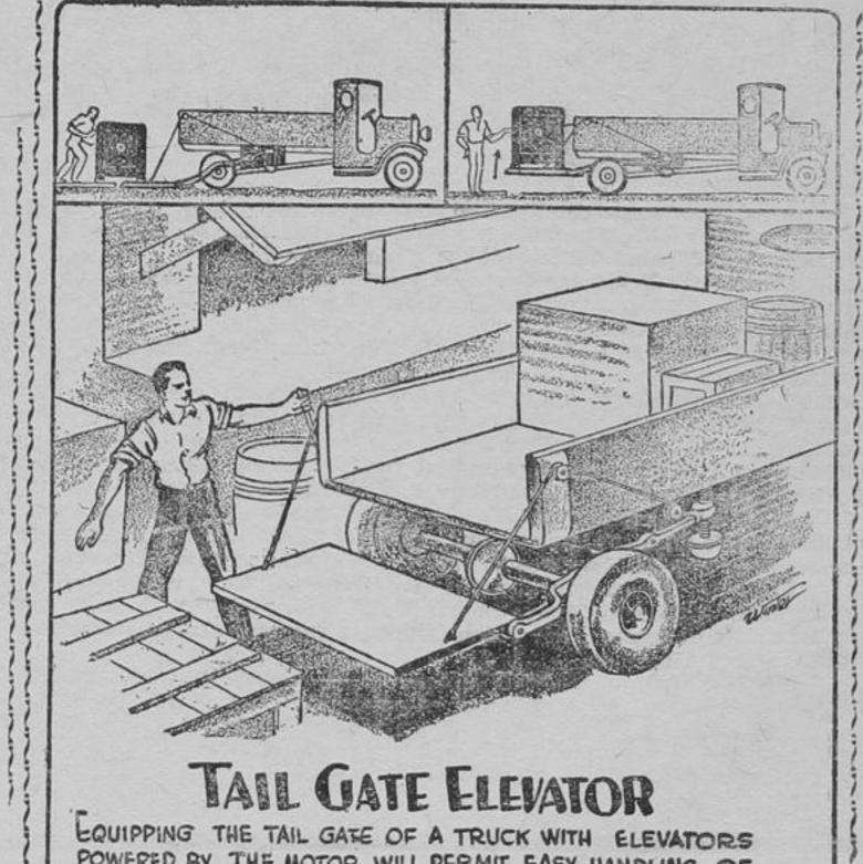
POWERED BY THE MOTOR WILL PERMIT EASY HANDLING OF HEAVY OBJECTS. CAN IT BE DONE?
