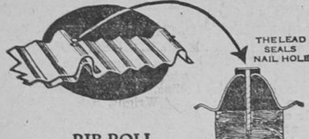
A "close-up" of Rib-Roll and the Preston Led-Hed Nail. Note the tight fitting, overlapping weather-proof joint. It is invisible from even a short distance away. Illustration shows the neat pattern which has been widely but unsuccessfully copied.
