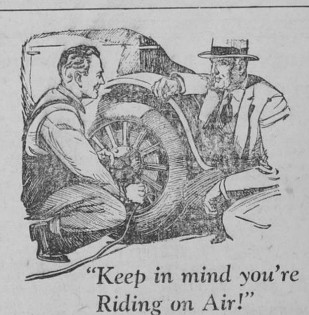
A IR lifts the load off the road. The heavier The the load the more air it takes. That's why tire makers have worked out the correct inflation pressure for every size of tire for different loads.
