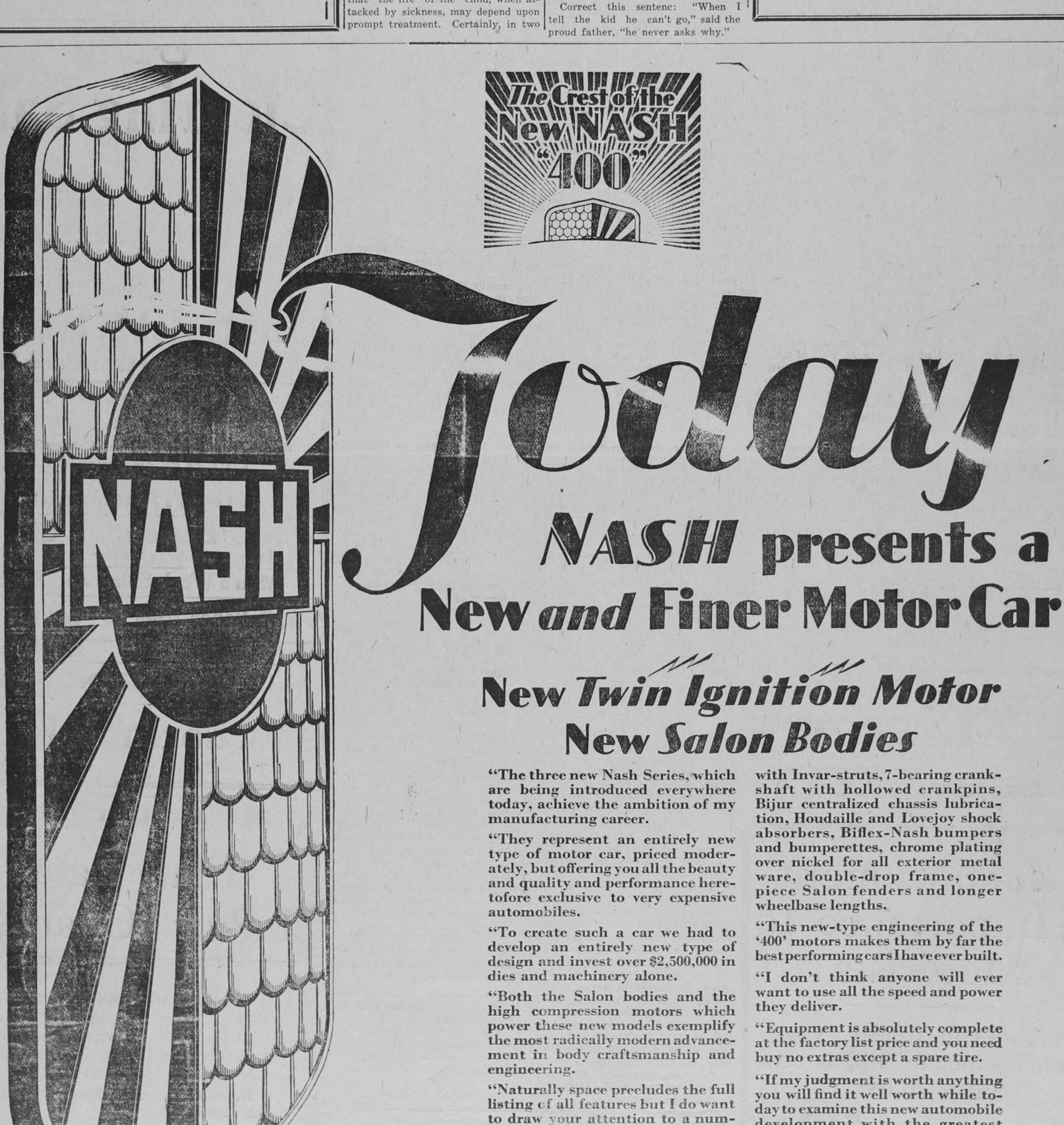
with Invar-struts, 7-bearing crankshaft with hollowed crankpins, Bijur centralized chassis lubrication, Houdaille and Lovejoy shock absorbers, Biflex-Nash bumpers and bumperettes, chrome plating over nickel for all exterior metal ware, double-drop frame, onepiece Salon fenders and longer
