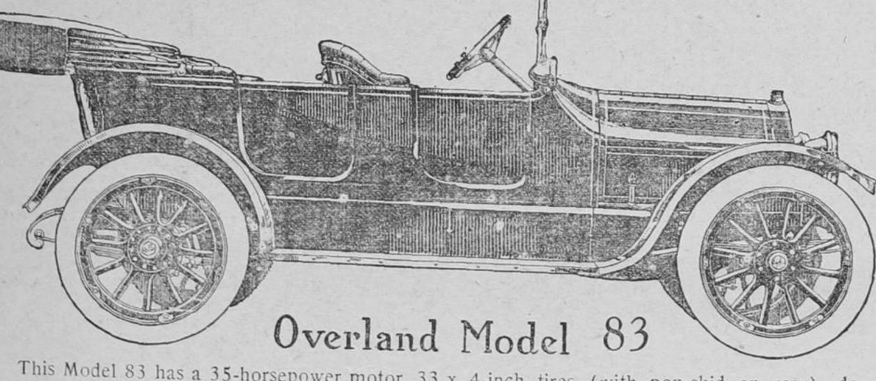
This Model 83 has a 35-horsepower motor, 33 x 4-inch tires (with non-skid on rear), demountable rims, collapsible windshield, one-man top, full stream-line body, with bell back, and bell cowl, demed mud-guards, dimmer headlights, 18-inch steering wheel, with electric control box on steering column.
