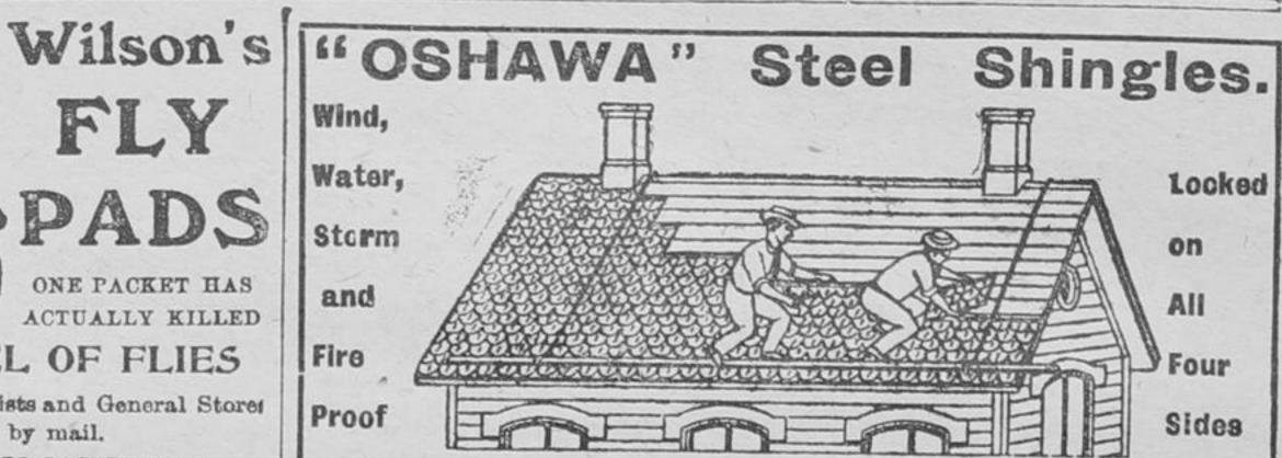
Made from Painted or Galvanized Steel, at prices varying from \$2.85 to \$5.10 per hundred square feet covering measure. This is the most durable covering on the market, and is an ideal covering for Houses, Barns, Stores, Elevators, Churches, etc. Any handy man can lay the "OSHAWA" shingles. A hammer and snips are the only tools required.
