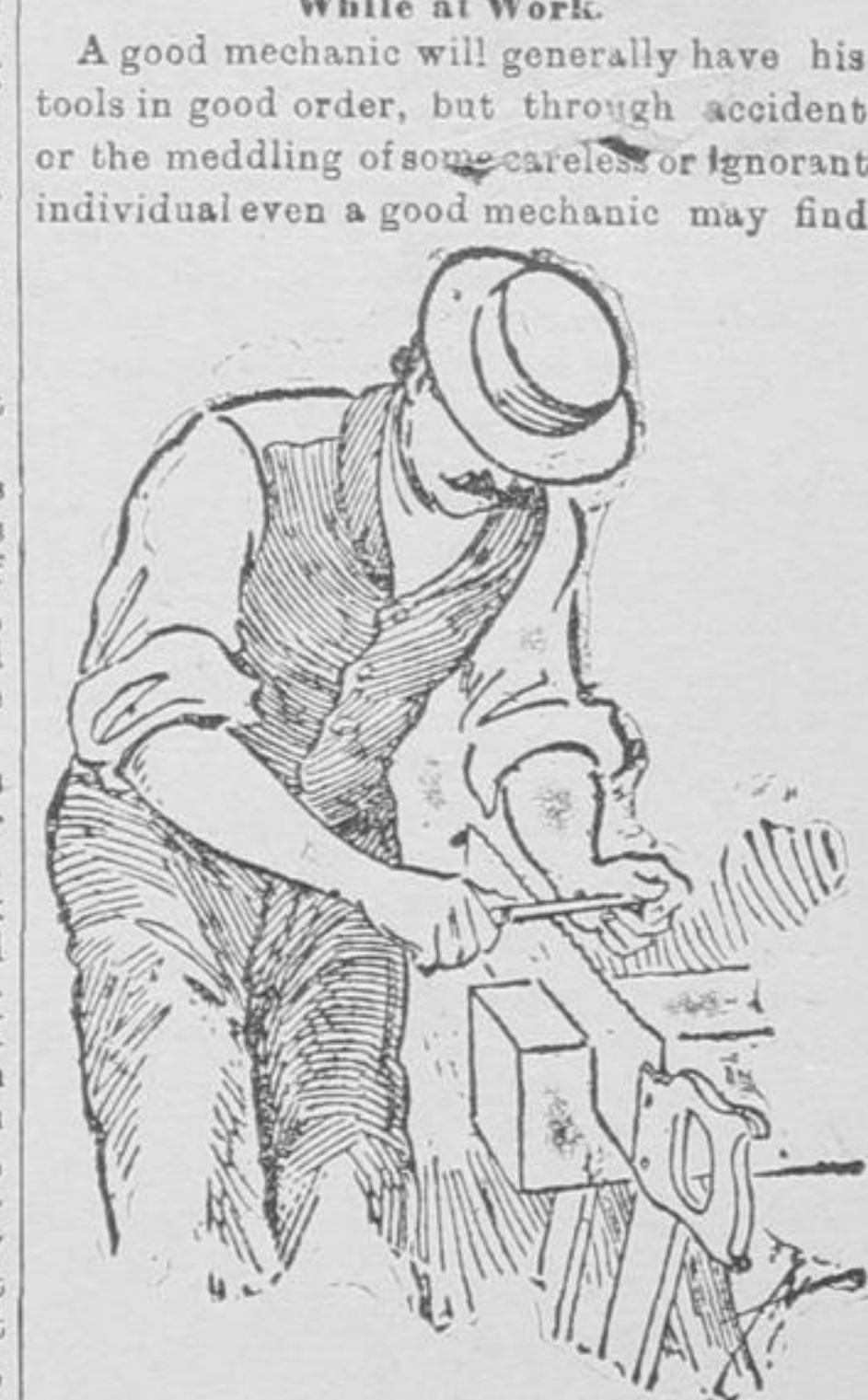
AN EXTEMPORIZED SAW VISE.
