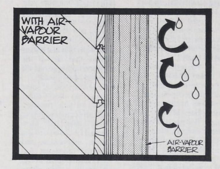
water-resistant barrier on the inside of a building shell accompanied by a breathable air barrier on the *outside* of the insulation to allow any penetrating indoor moisture to escape.
