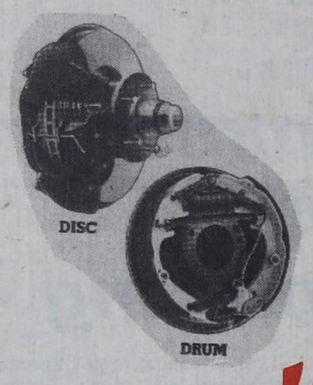
Brakes should be inspected every 24,000 kilometers or once a year. Inspection should include master cylinder, fluid levels, lines and hoses, pads and linings, drums and rotors. Worn parts should be replaced.
