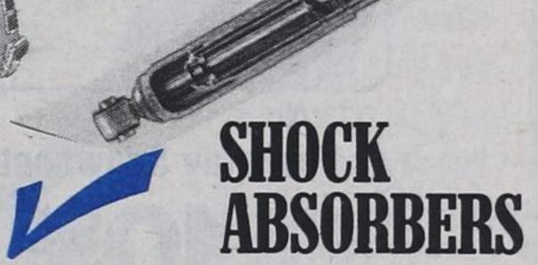
Shocks should be examined every 18,000 kilometers for signs of fluid leaks or bushing and mounting wear. Worn shocks can cause difficult handling, bottoming out, sagging springs or uneven tire wear.
