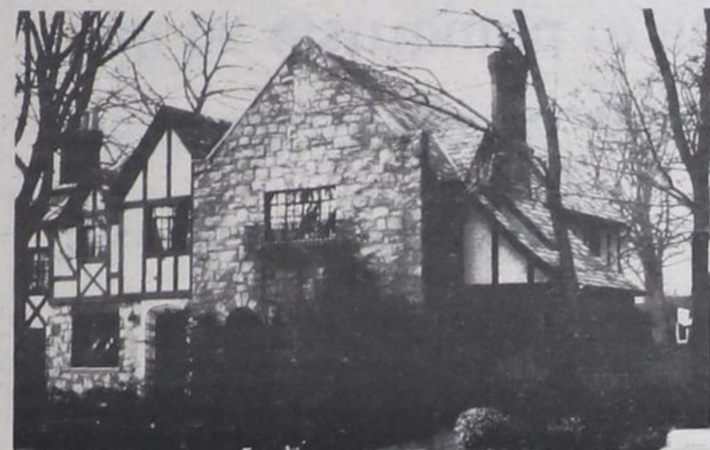
Tudor with molded stone trim around doorway at left, diamond-paned windows, tall protruding chimney pots, and stone facing.
