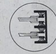
Double insulation by wool pile weatherstrip on both sides of glass sash.
