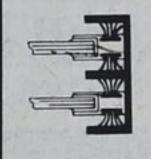
Double insulation by wool pile weatherstrip on both sides of glass sash.
