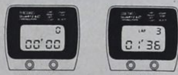
00'00 The stop/start button is used to start and stop the stopwatch.
