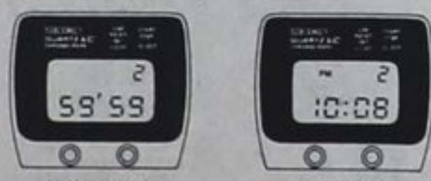
55'55 The stop/start button is used to start and stop the stopwatch.
