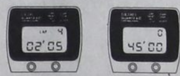
02'05 Press and hold the stop/start button to start the stopwatch.
