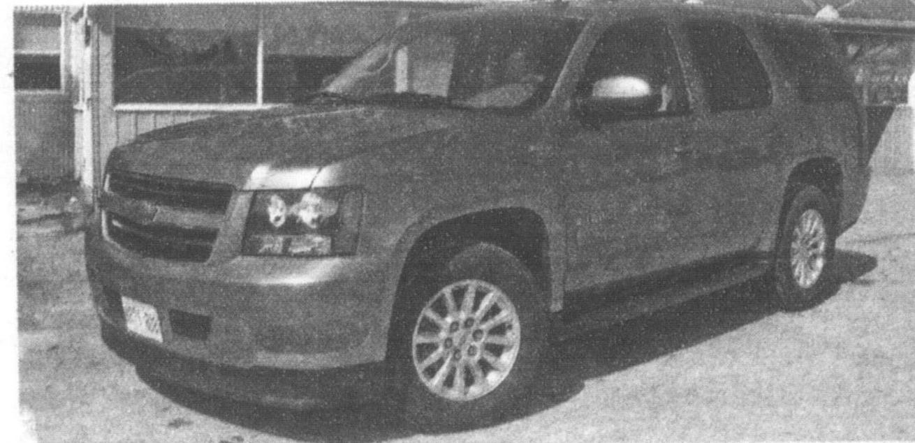
It ain't easy being big and green, the 2-mode hybrid in the 2008 Chevrolet Tahoe Hybrid full-size SUV saves up to 25 per cent on fuel consumption by running on battery power, gasoline engine or a combination of both.
