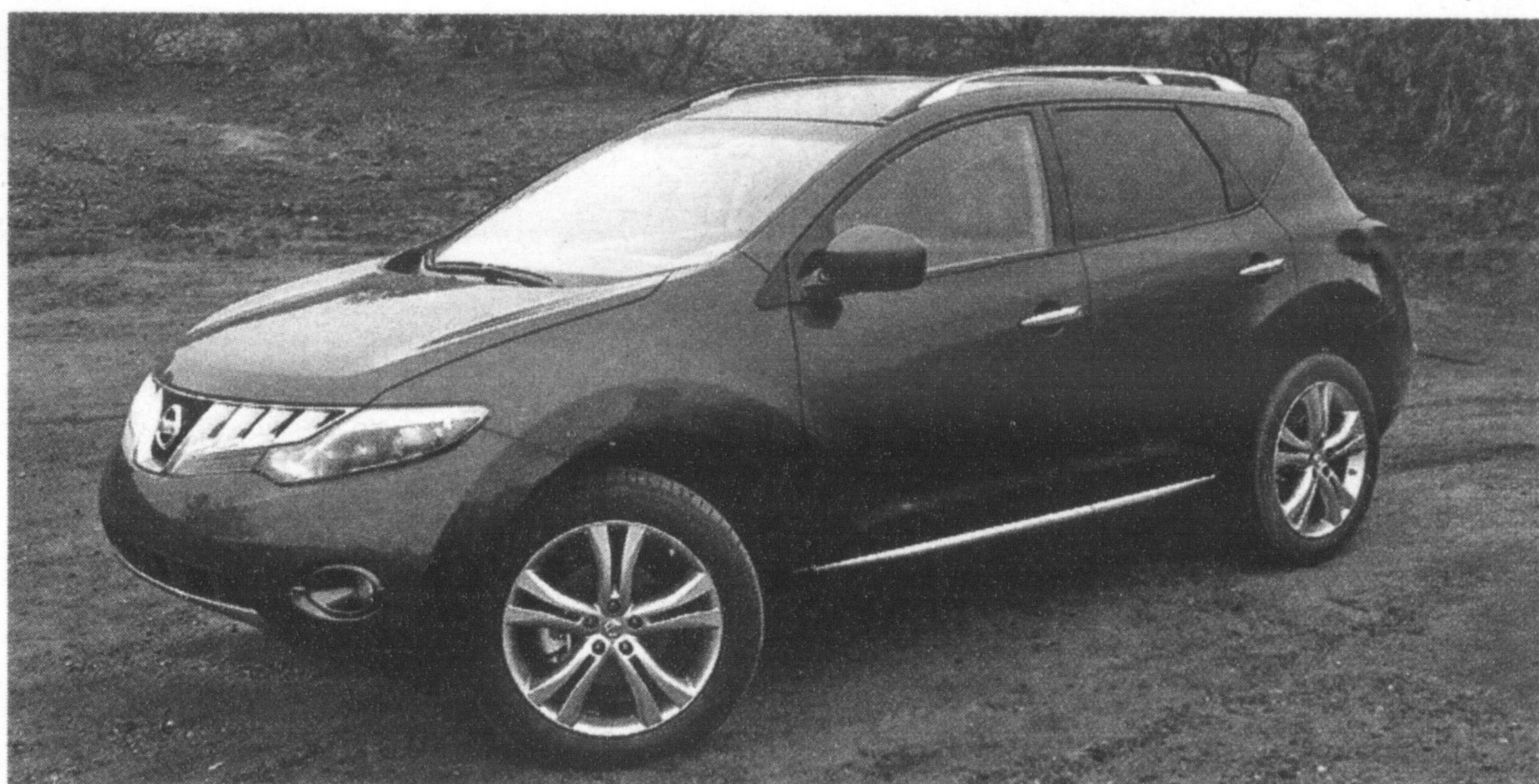
The 2009 Nissan Murano looks similar on the outside but it has undergone an extensive redesign that includes a new chassis, all-wheel-drive system, suspension and CVT transmission that sharpens steering response and handling especially in adverse conditions.
