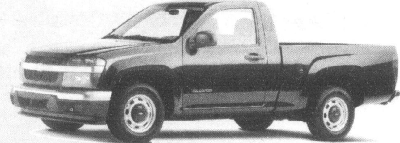
175 HP Vortec 2800 DOHC Engine • ABS • 5 Speed Manual • 2 Position Locking Tailgate • 15" Wheels • 2WD
