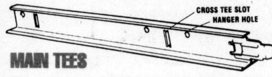
The metal framing members of your ceiling grid are called "tees". Main tees are hung from above by hanger wire. They run between the wall angles and form the support for the ceiling.
