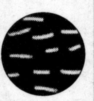
Textile fibre mini-studs improve road grip and tread durability for 'studded' tire performance without studs.
