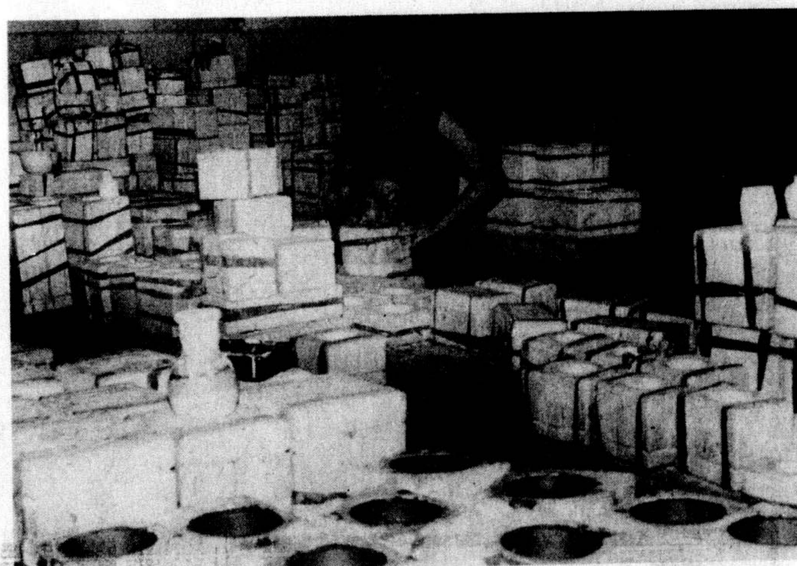
FILLING MOULDS with clay is the job of Mae Chaisson. When the clay is set Mae removes the elastic bands and carefully parts the still-wet casting.
