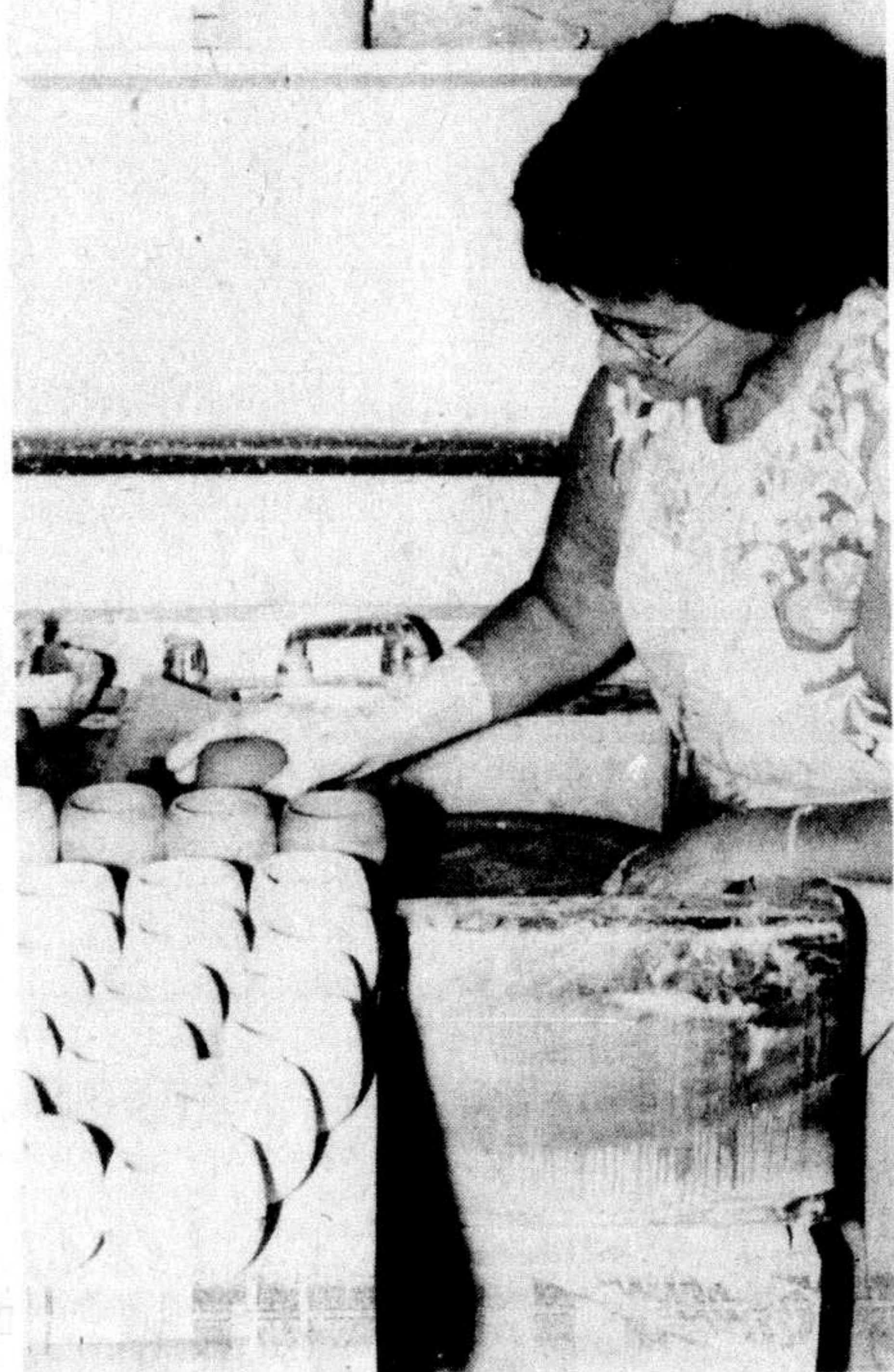
ELSIE JOYCE makes the top of a mug level by dipping it into water and rolling it gently on a flat surface.
