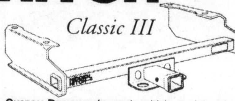
CUSTOM DESIGNED for each vehicle model and HEAVY DUTY TOWING CAPACITY can tow up to 6,000 lbs. gross towing weight, 600 lbs. tongue weight. The towing capacity may be increased up to 10,000 lbs. G.T.W., 1,000 lbs. T.W. when using a weight distribution system. A typical application is used for towing utility trailers, boats, R.V.'s or horse trailers. Limited Lifetime Warranty.
