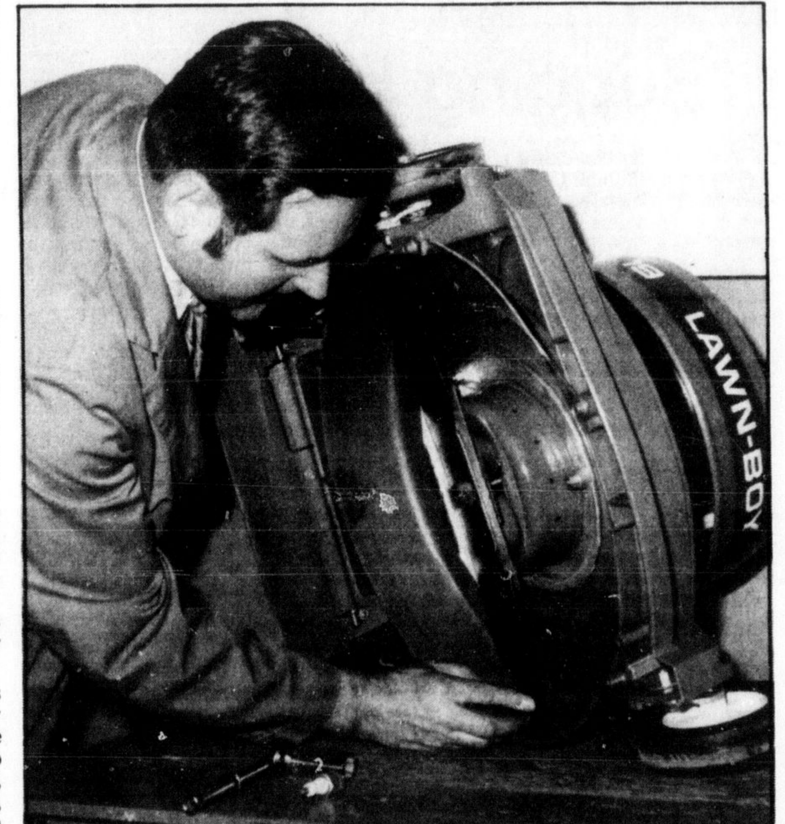
WHEN TUNING UP your lawn mower for this summer, check the blade. If it is badly nicked or bent, follow the directions in your owner's manual to remove it, then take it to a dealer or service centre for sharpening and balancing, or replacement.
